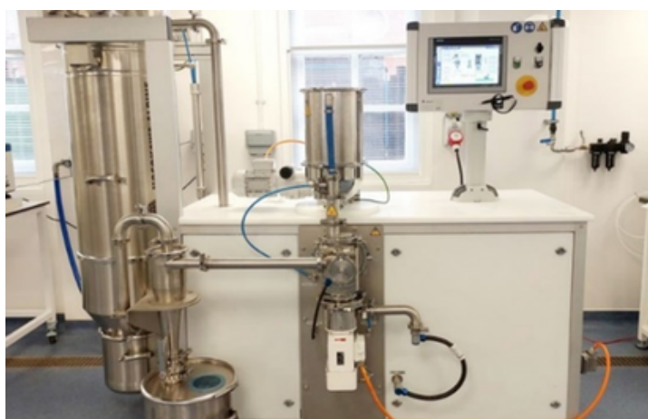
The Hosokawa Alpine Dry Fractionator can generate two key fractions from legume & cereal flours without the need for water, chemicals or solvents.
